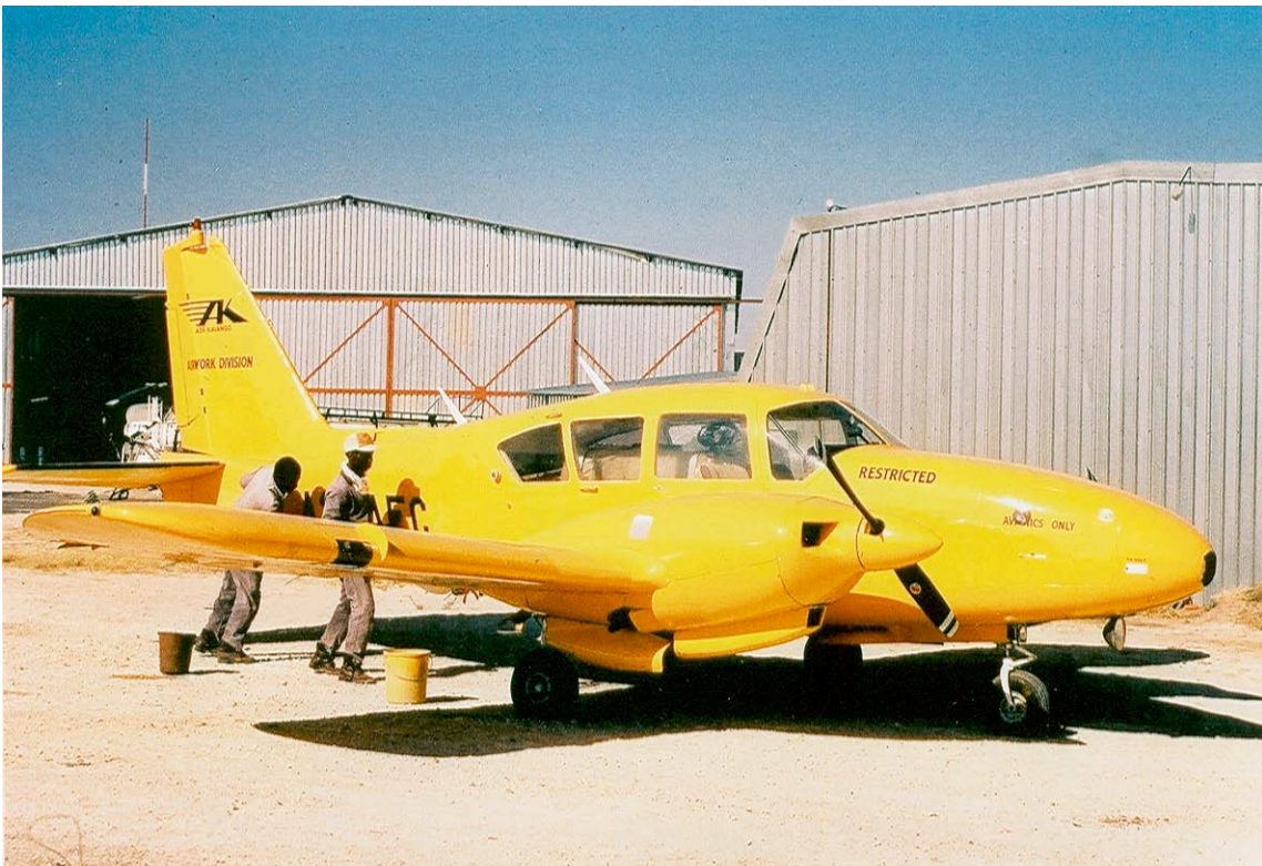
Photo 60. A modified fixed wing aircraft used for aerial spraying of insecticides to control the tsetse fly in the late 1980s and early 1990s.
